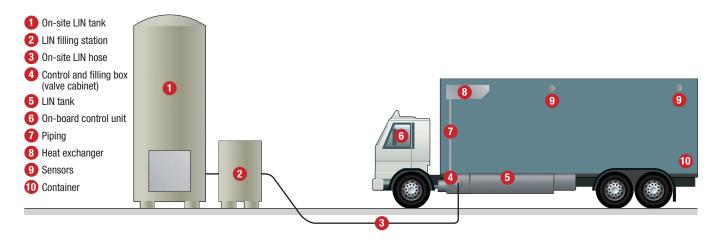
Frostcruise: a greener approach to onboard truck refrigeration to adopt a similar approach for its larger refrigeration models, but it is far from straightforward on bigger trailers. "The problem is that refrigerants are extracting heat from a place where it is not wanted, but the power and capacity have to come from somewhere," he reasons. "We are looking for solutions, but nothing is likely in the next 12 months."
